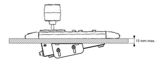
The drawing shows the mounting position of the fixation brackets.
